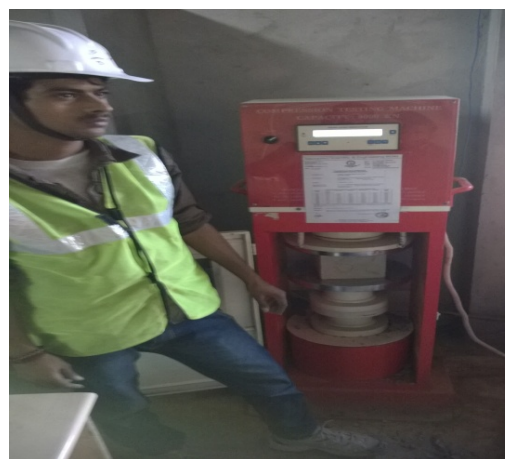
Fig. 6: Testing of Cubes
