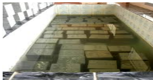
Fig. 5: Curing of cubes
