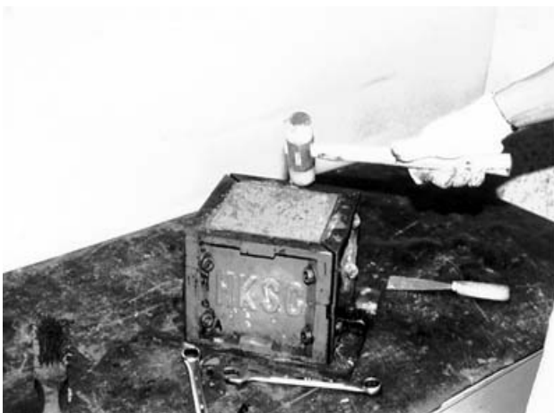
Fig. 4: Demoulding the Test Cubes
